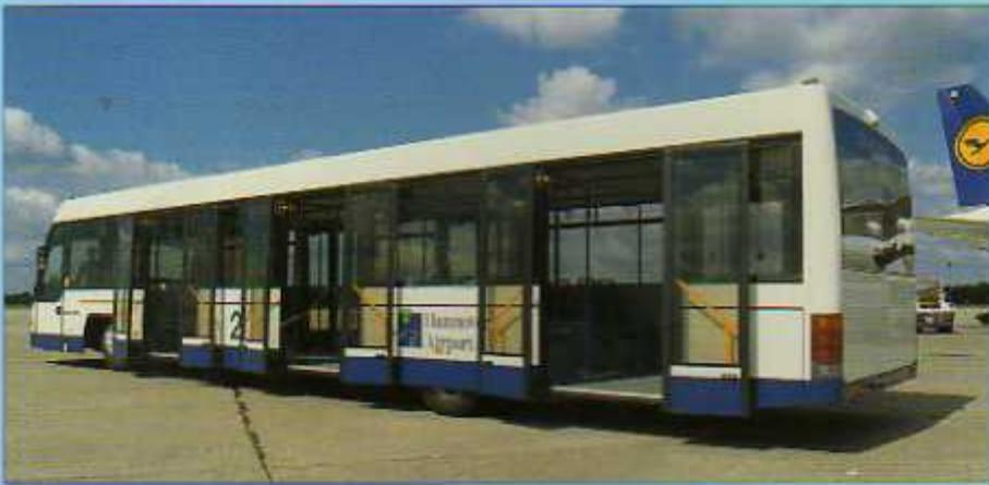
*Maximum comfort and extremely short load-unload cycles are due to the 3 extra-large doors on each side and the suspension lowering ability of the COBUS for easy embarking and disembarking.*
