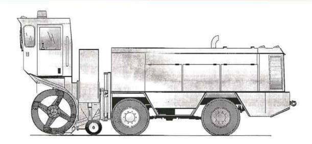
The Stewart & Stevenson RSS-1250 Cabover unit is a single engine, 4000 tons per hour performance machine. The vehicle is hydrostatically driven, while the blower head is driven mechanically through the Allison power shift transmission. This thoroughly engineered drive system provides the RSS-1250 with maximum horsepower utilization for the demanding task of snow removal. User's gain an excellent performance to weight ratio with the compact and maneuverable RSS-1250.
