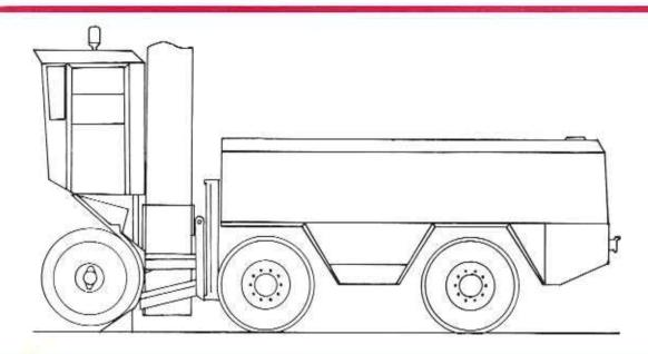
The Rolba/S&S RSS-1000 Cab Over Plow unit is a 3000 T/H capacity, single engine performer. The carrier is hydrostatically driven with a mechanically driven blower head run through a 4-speed Allison automatic transmission. This effectively engineered drive system provides the Rolba/S&S RSS-1000 Cab Over Plow with maximum horsepower utilization for the demanding task of snow
